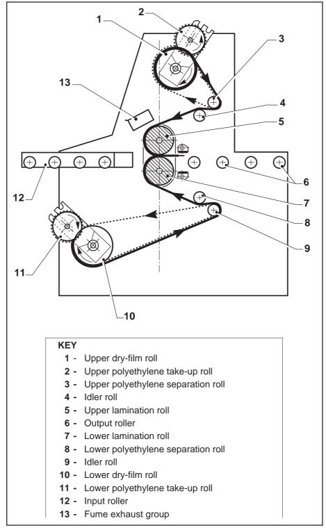
Fig. 11 - DRY-FILM AND POLYETHYLENE THREAD-UP
