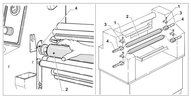
Fig. 15 - REPLACEMENT OF LAMINATION ROLLS
