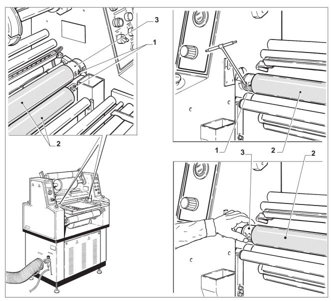
Fig. 14 - REPLACEMENT OF LAMINATION ROLLS
