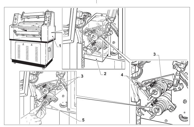
Fig. 13 - REPLACEMENT OF LAMINATION ROLLS HEATER
