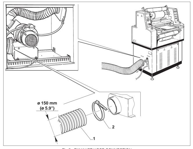
Fig.5 - EXHAUST HOSE CONNECTION
